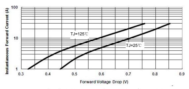
Fig.3-Typical Instantaneous Forward Voltage Characteristics
